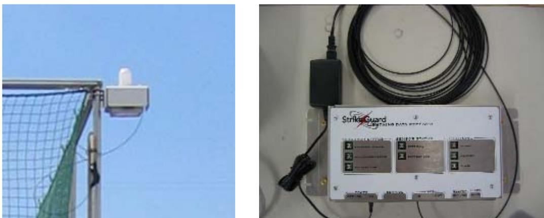
Fig. 1: StrikeGuard Sensor (left) and Receiver (right)
