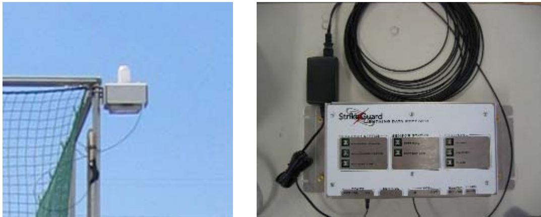
Fig. 1: StrikeGuard Sensor (left) and Receiver (right)
